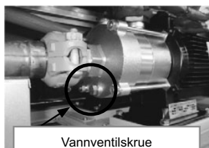
Vannventilskruer (Maks. to omdreininger)
